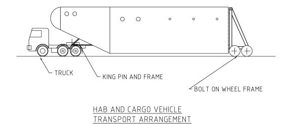
Figure 12. Transportation mode of MARS-OZ modules, using detachable wheels and a prime mover. Two such prime movers will be required to set up the base on the chosen site.
