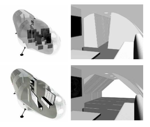
Figure 7. Interior schematics of the MARS-OZ Hab module showing representative different configurations allowable with movable bulkheads and fittings as developed by Kirtsen Thompson Architects, Melbourne. TOP LEFT: control cabin in "cockpit" configuration. BOTTOM LEFT: control cabin in "conference" configuration. TOP RIGHT: View aft on upper deck showing all eight sleeping cabins deployed. BOTTOM RIGHT: view aft showing all sleeping cabins folded away.
