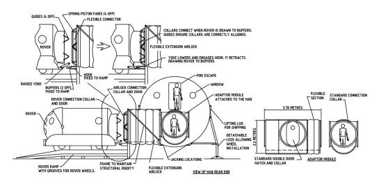
Figure 9. View of Hab rear, adaptor module and flexible extension airlock and rover docking system.
