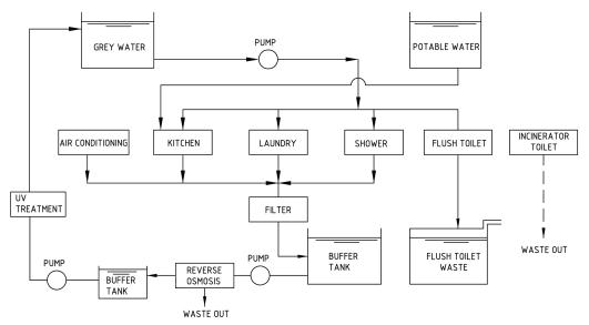
Figure 10. Diagram of the water recycling system
