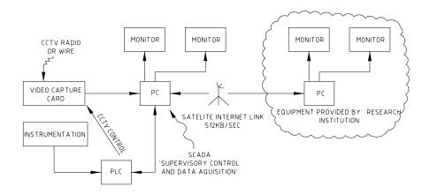
Figure 11. Diagram of the data collection and communication system
