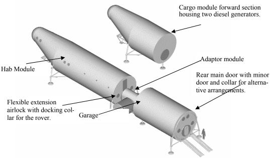
Figure 5. The MARS-OZ base configuration. Showing habitat module (left), adaptor and airlock module (centre) garage module (bottom left) and power and simulated ascent stage housing (top).
