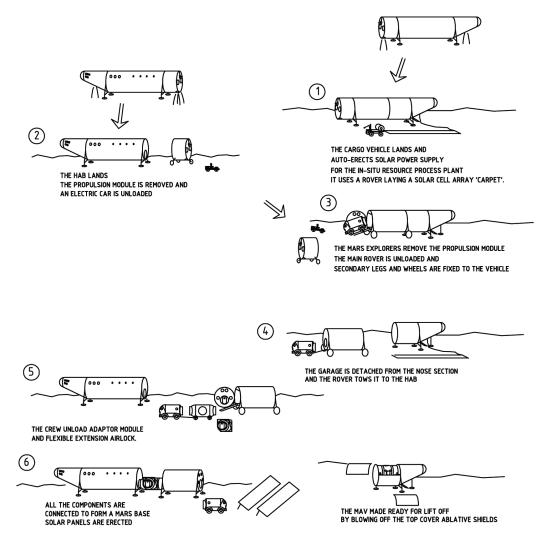
Figure 4. The Assembly of the base on Mars.
