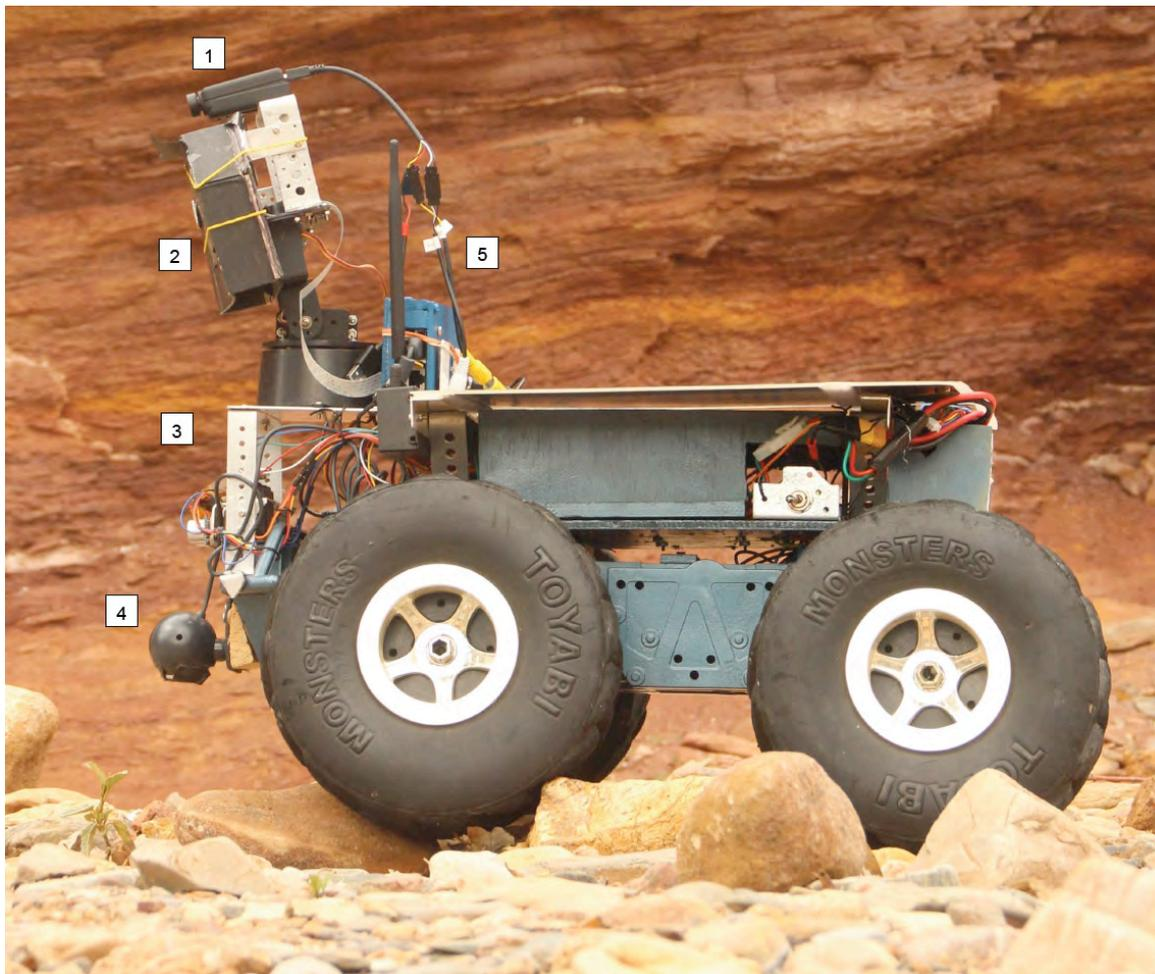
*Fig. 1 Overview of Main instruments carried on Little Blue: (1) FPV navigation camera, (2) MMC, (3) Non-contact thermometer swing arm bay (4) Webcam for macroscopic*
