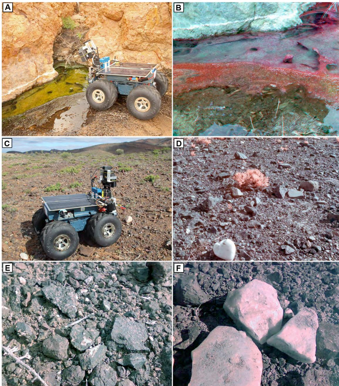
*Fig. 3. (A) Little Blue at the hot spring. (B) False-colour view of the hot spring from the MMC. Photosynthetic algal mats are revealed as red in NIR. (C) Little Blue undertaking tests to identify hypoliths at Arkaroola, one of which is immediately right of the rover. (D) False-colour image from MMC of hypolith shown in part A. (E and F) Images of ground and hypoliths from the Little Blue webcam*
