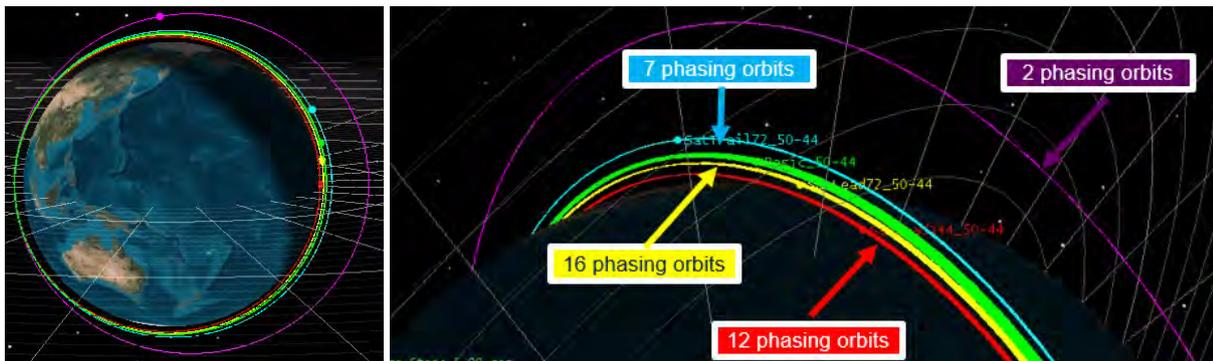
Fig. 7a & 7b: A typical MDO-generated optimal solution (note the Trailing 144° satellite’s phasing orbit relatively large size compared to its counterparts (purple line) and the base orbit is marked in green)
