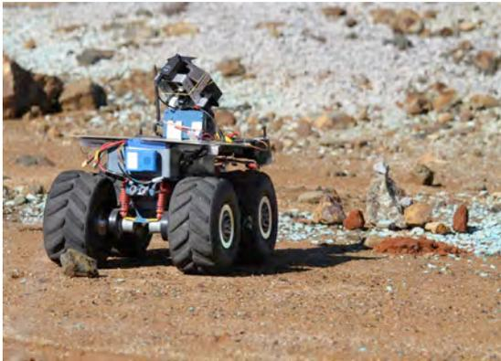
Fig. 6 Current Marsobot's testing on McGuirk mine
