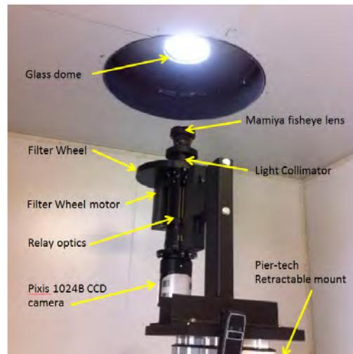
Figure 1: The airglow imager and filter wheel setup in the TRACE container
