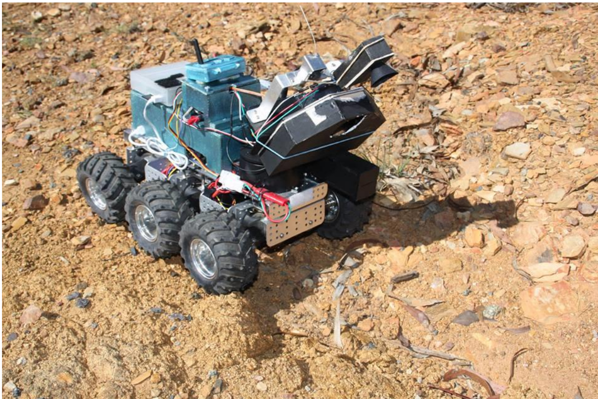
Marsobot Junior , a 7 kg robot, built by Steve Hobbs of MSA is equipped with web cams, multispectral camera, spectrometer and a non-contact thermometer. It will be tested in the hot springs and volcanic terrains of New Zealand.
