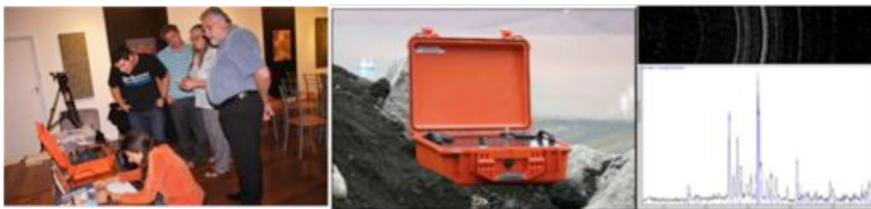
Figure 4.3.5: Left: the miniCheMin field instrument displayed during an EPO event organized at the art gallery in Port Headland. Autonomous operation 14.5kg with embedded batteries and computer (45x32x12cm); Right Rosalba Bonaccorsi foreground.
