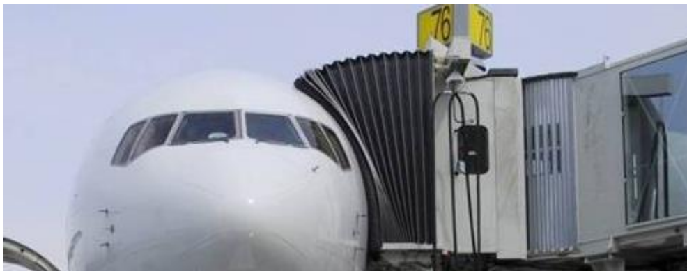
Figure 4.4.6 The picture of Boarding bridge awning
