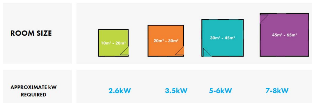
Figure 4.2.2 Room size and power required
